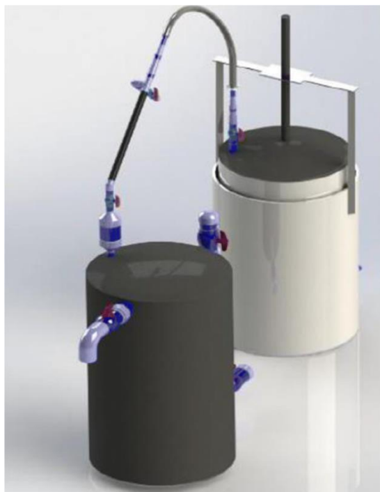
Fig. 3. Model of the digester and storage tank
